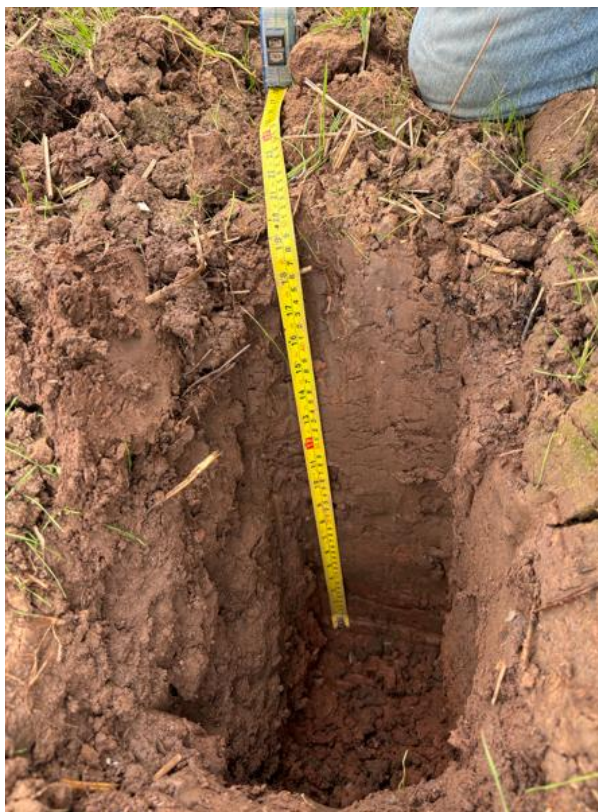
Photos 4 and 5: Subgrade 3a in Parcel 79, reddish fine loamy soils
