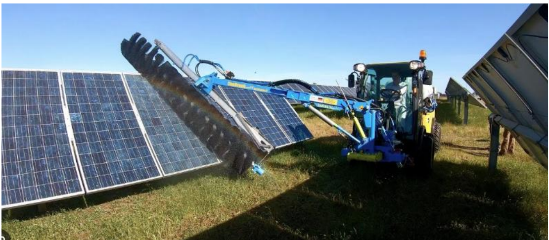
Photo 48: Cleaning of Solar Arrays
