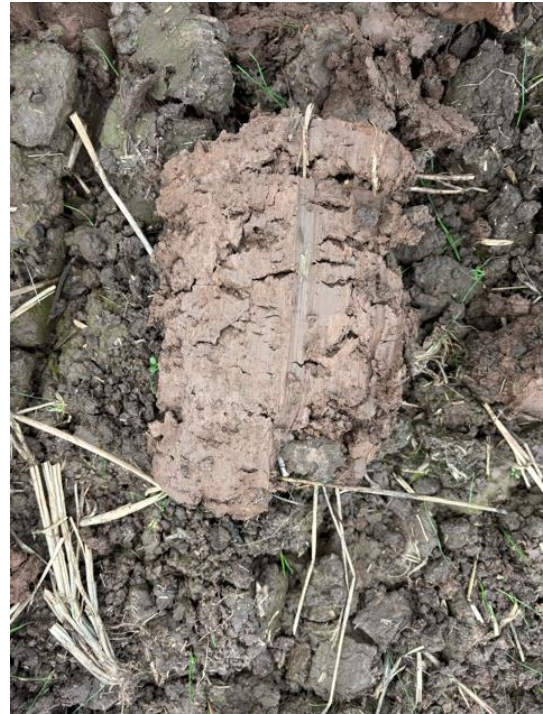
Photos 6 and 7: Subgrade 3b, Parcel 199, reddish clayey soils affected by groundwater
