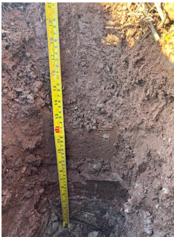
Photos 4 and 5: Subgrade 3a in Parcel 79, reddish fine loamy soils
